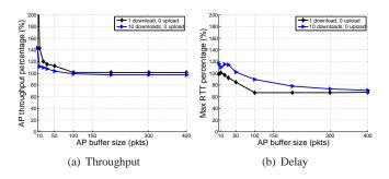
Fig. 19. Performance of the  $A^*$  algorithm for 802.11 DCF operation when there are download flows only in the network. Here we illustrate the percentage (between the results achieved using the  $A^*$  algorithm and those using varied AP buffer sizes as shown on the x-axis) of both throughput and delays. Physical layer data and basic rates used are 54 and 6 Mbps.
